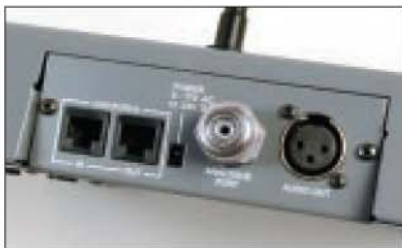
CDPM with analog interface installed. (One mic in the system needs an analog interface)
